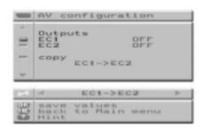
Once the copy direction has been set (e.g. EC1 → EC2), the outputs of the appropriate SCART sockets will switch to OFF. If EC1 or EC2 are set to OFF, this means that no TV output signals will be directed to the SCART socket.
